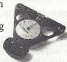
We use this special gauge to insure optimal spoke tension.
